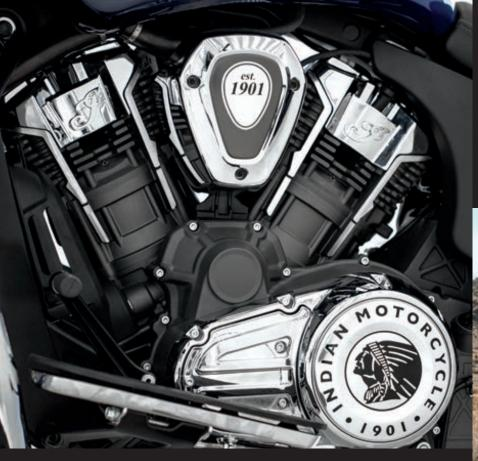
Our all-new liquid-cooled PowerPlus V-twin is the most powerful engine in its class. With overhead camshafts and four valves per cylinder delivering a blistering 122 hp and 128 ft-lbs of torque, it redefines American performance. With inverted forks and a hydraulically adjustable Fox monoshock, radial-mounted Brembo brakes, full LED lighting, and Standard, Sport and Rain ride modes, the Indian Challenger is fully loaded with features to improve your riding experience.
